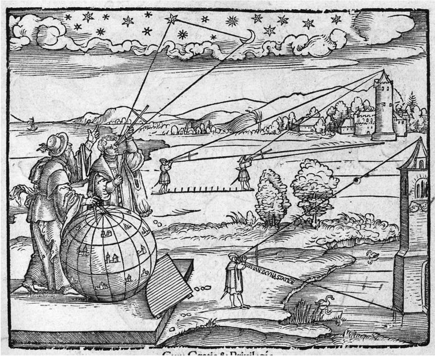
Figure 1. The use of the cross-staff in astronomy and the measurement of buildings. Title-page woodcut from Peter Apian's Introductio geographica in doctissimas Verneri annotations (Ingolstadt, 1533). Copyright Alamy.
